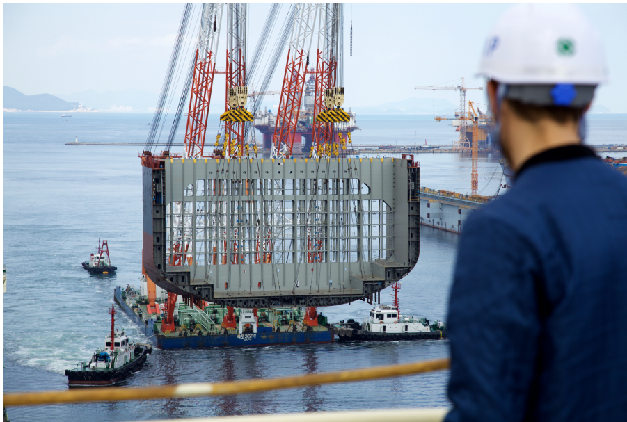
Figure 6: Lift of a parallel midship mega block of a Triple-E container ship.
